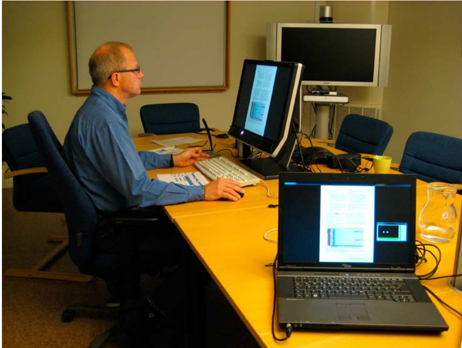
Figure 6-3. A typical setup in an eye-tracking experiment. The participant sits in front of the monitor, and the experimenter observes on a remote desktop.
