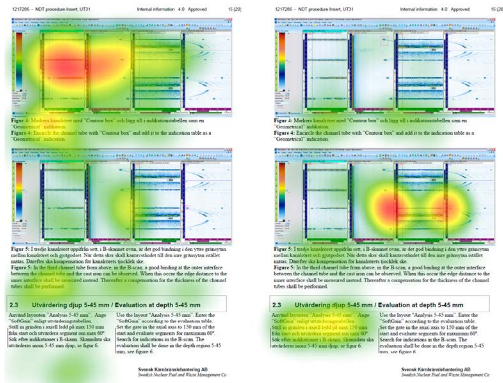
Figure 6-7. Heat maps showing the fixation count (red areas indicate higher fixation count) of a participant with a scattered search pattern (i.e. who is struggling with the task and not understanding how to carry it out; left) in contrast to a participant engaging in a targeted search (right).
